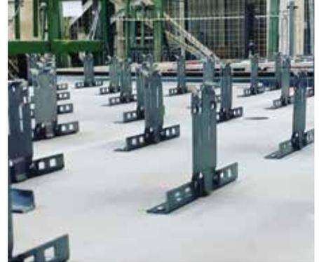
**Fig. 3:** VST wall formwork is assembled from three key components: 24 mm (nearly 1 in.) thick cement-bonded particle boards, clip angles, and spacers. The clip angles are attached to the facing panels by a computer-controlled drilling machine that ensures precise spacing. Spacers lock into slots in the clip angles and precisely set the wall thickness
