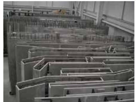
**Fig. 4:** Completed VST wall formwork can include unique bends and end closures
